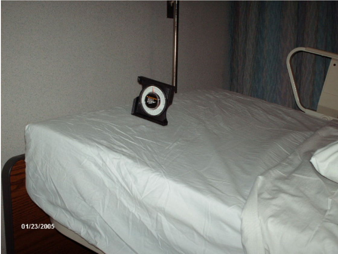
Figure 6 Placement of Pitch and Angle Locator
